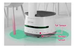
The 3D camera sensor detects low obstacles, while ToF sensors reliably recognize nearby or rapidly approaching objects, allowing ServeBot to avoid even small obstacles as it safely and autonomously navigates the spaces.
